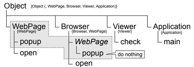
**Fig. 2** Example: Locality of Changes. Gray boxes indicate classes and their extensions, sets enclosed in curly braces indicate the scope of a class. Classes enclosed in parentheses account for hierarchical scoping.
