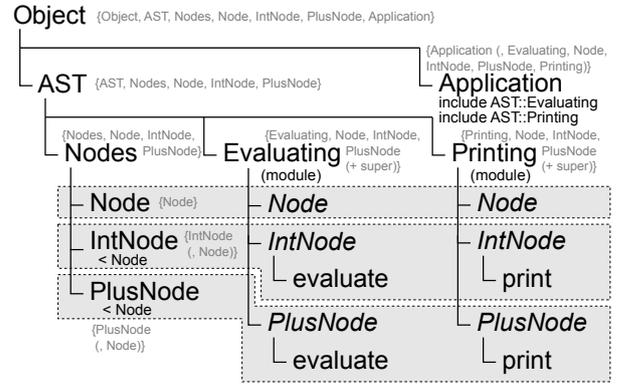
**Fig. 5** Example: AST Library. Classes enclosed in parentheses in scope sets account for inheritance scoping.
