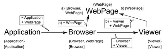
**Fig. 3** Example: `Browser` uses `Viewer`. Sets enclosed in curly braces indicate the scope of a class (see Figure 2). Sets enclosed in square brackets indicate class activation sets after calling a method (specific to this scenario). Arrow annotations indicate add/remove operations to the class activation set.
