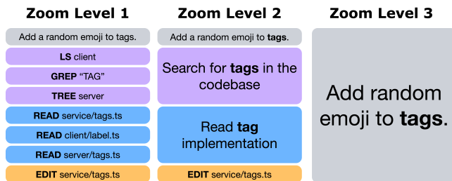
Figure 5. Conceptual figure of our implementation of semantic zoom at three levels. As the developer zooms out, individual context nodes are replaced by LLM-generated summaries, and groups of summaries are themselves summarized into higher-level overviews.
