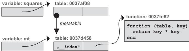
Figure 3: Example where `_index` is used to return the squared value of the accessed key (field).
