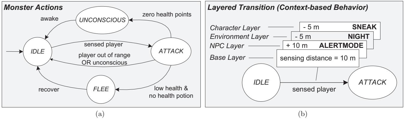
Figure 2: State transition diagram with actions of a monster and behavioral variations.
